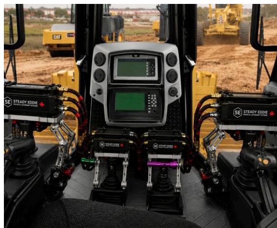
A DOZER'S OPERATOR STATION. THE DOCK IS FITTED ONCE, MECHANICALLY. EVERY CAB IS DIFFERENT; THE UNIT IS THE SAME
